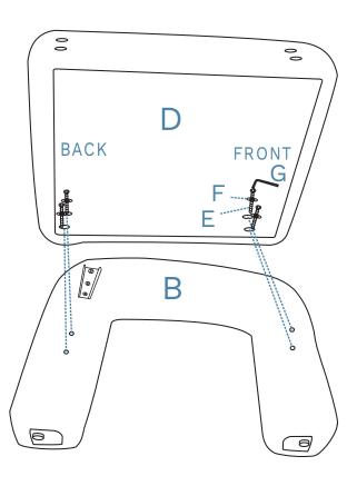
Attach 1 x cushion (D) to 1 x leg (B) and secure with 4 x screws (E) and 4 x washers (F). Tighten with an Allen Key (G).
