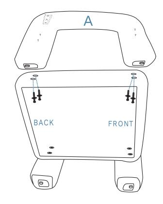
Attach 1 x leg (A) to assembled frame as shown and secure with 4 x screws (E) and 4 x washers (F). Tighten with an Allen Key (G).
